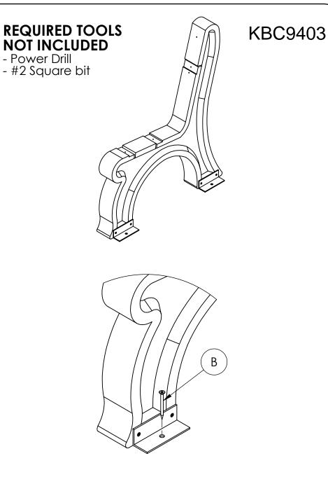
**Step B** Screw 2" screws (C) into mounting surface.
