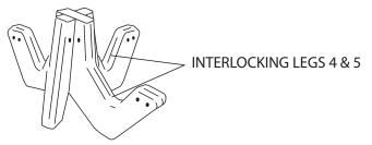
Attach seat-to-leg brackets (6) to interlocking legs (4) & (5) with 3/8" x 5 1.2" hex flange screws (8) with locking hex nuts (9) and washers (12). **LEAVE SCREWS LOOSE.**
