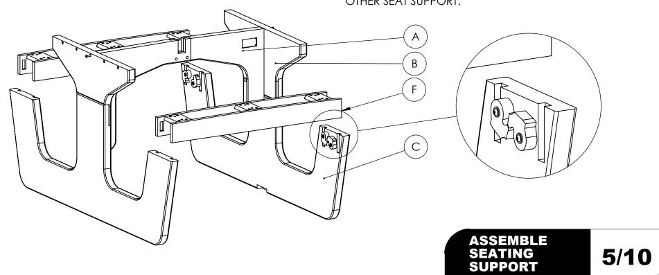
**STEP THREE:** ATTACH THE ENDS OF THE TWO GUSSETS (A) TO EACH OTHER USING 3/8" BOLTS (J), FLAT WASHERS (K), AND LOCKING NUTS (L). RUN NUT ONTO BOLT BUT DO NOT TIGHTEN FULLY YET.
