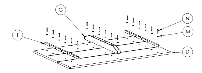
**STEP SIX:** PLACE TABLE TOP ASSEMBLY ONTO TABLE. CAREFULLY TAP INTO PACE WITH A RUBBER MALLET IF NECESSARY TO ALIGN HOLES. START EACH 1/4"-20 MACHINE SCREW (N) OR (P) A FEW THREADS BEFORE GOING BACK TO TIGHTEN ALL OF THEM. USE 1/4" FLAT WASHER (M) WITH EACH SCREW AS SHOWN.
