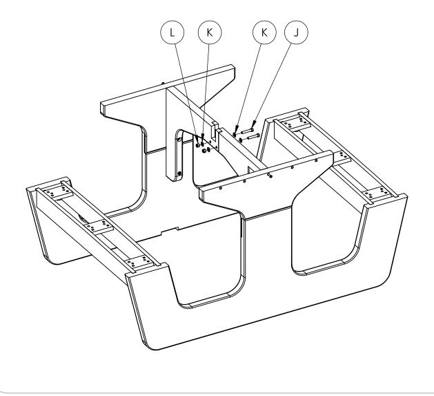
**STEP FOUR:** WITH HELP FROM ANOTHER PERSON, ROLL THE TABLE UP ONTO ONE OF IT'S ENDS. WITH ONE PERSON HOLDING THE TABLE STEADY, ATTACH THE LOWER LEG BRACE INTO THE NOTCHES AT THE LOWER EDGE OF THE END FRAMES. MAKE SURE THE COUNTERSUNK HOLES FACE OUT. ATTACH USING (4) #10 X 2-1/2" FLATHEAD SCREWS (S). HAND TIGHTEN. **DO NOT USE POWER TOOLS.**
