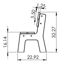
Recycled Plastic Concrete Powder Coated Steel
