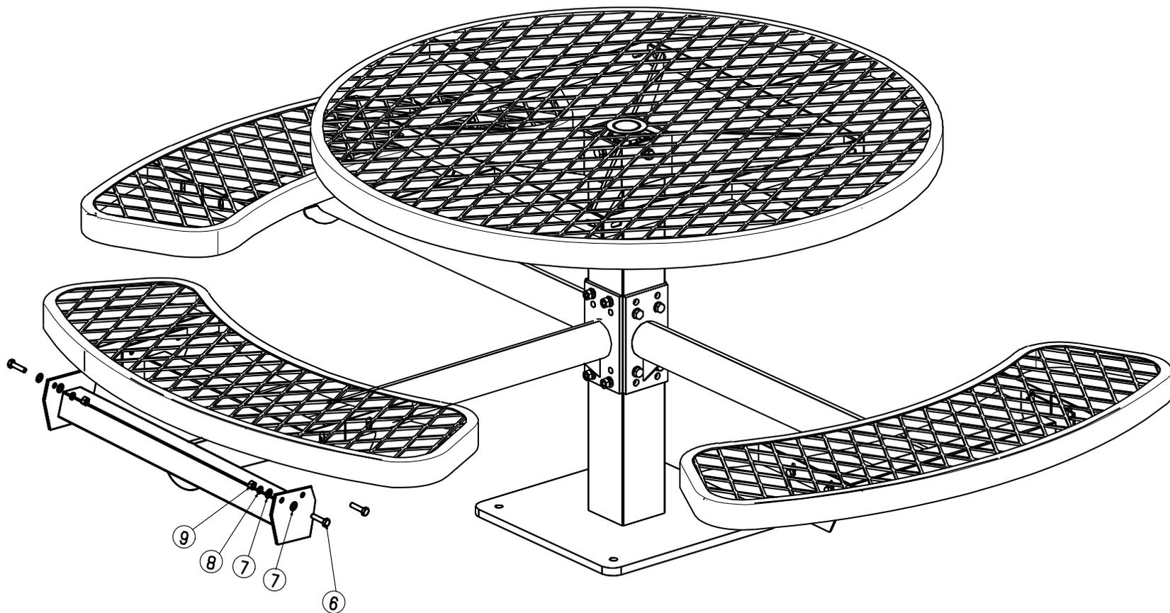
Attached the seat tops to the side frames using the specified hardware.
