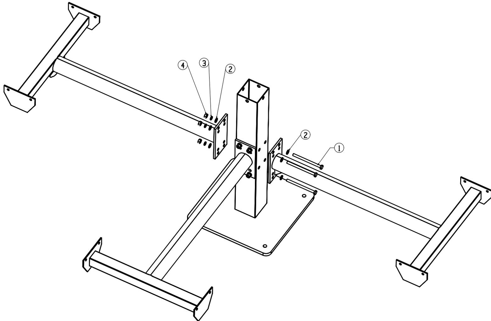
Attach the side frames to the pedestal frame using the specified hardware.
