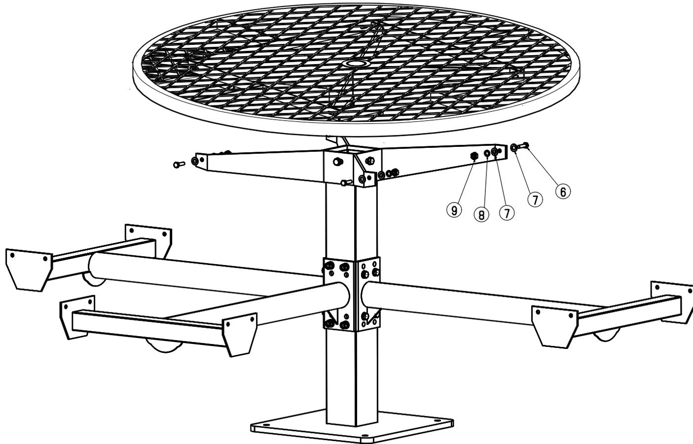
Attach the table top to the table support bracket using the specified hardware.
