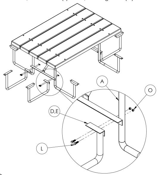
STEP 5: Attach Pipe Frame ClampsAt the base of the table, place a pipe frame clamp (J) around each side of the end support
